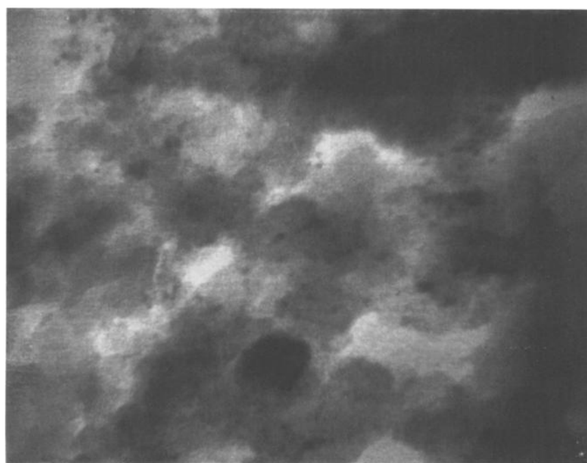
Fig. 3. STEM picture of Pd/CeO 2 -SiO 2 prepared by photodeposition.
